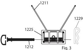
Step 2: Using the adjustment pin attach the tire stop to the front post
