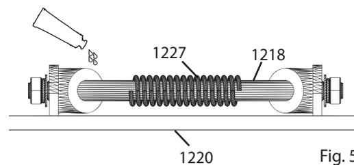
Step 4: Lubricate the pivot points of the cradle before use
