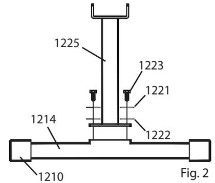
Step 2: Using the adjustment pin attach the tire stop to the front post
