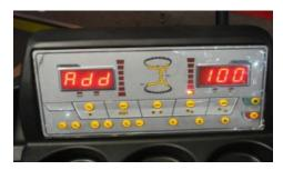
10) Manually rotate the wheel until all indicating lights on the "outer" side of the display are fully illuminated and then add the 100g calibration wheel weight to outside of wheel at the 12 o'clock position
