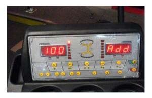
12) Remove the 100g weight from the outside of the wheel
