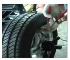
13) Rotate the wheel until all the indicating lights on the "inner" side of the display are fully illuminated and then add the 100g calibration wheel weight to the inside of wheel at the 12 o'clock position
