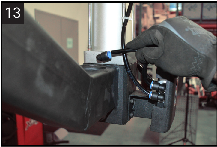
Connect airline from Switch Panel(#5) to cylinder fitting.
