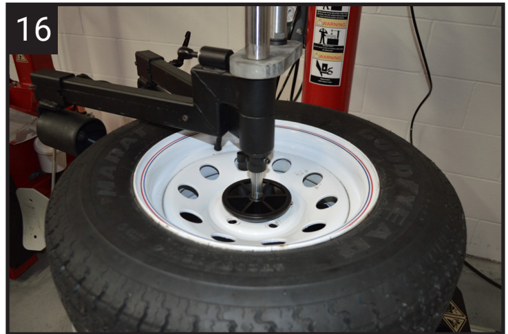
Press toggle switch on the Switch Panel(#5) down until the Centering Cone(#13/14) meets the center hub of the wheel.
