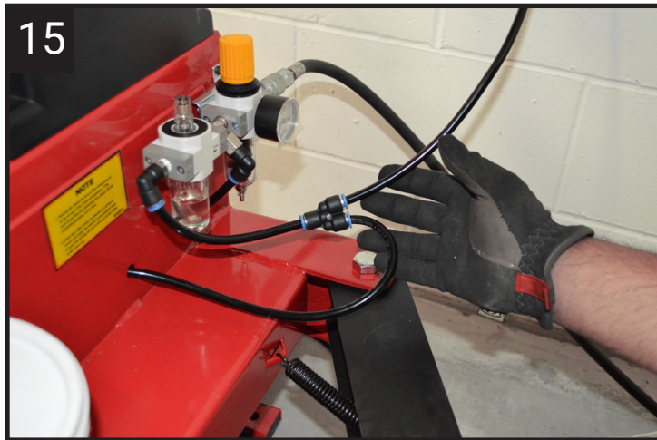
Connect Airline Y Fitting(#9) to airlines on TC-450S machine.
