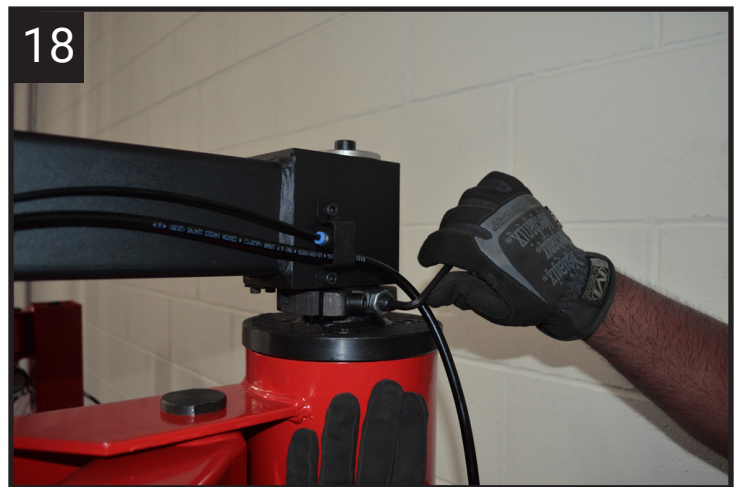
Tighten the two 8mm studs on the Lock Collar(#6), then tighten the jam nuts. *These last two steps ensure that the pneumatic lock built into the Assist Arm Assembly(#1) will engage when the arm is centered over the wheel.
